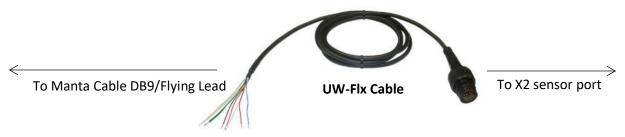
UW-Flx to Manta DB9/Flying Lead cable wiring. All unlisted signals are not-utilized and should not be wired to the X2.
